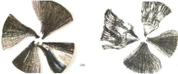
Figure 3: Chips formed when drilling Grade 3 ADI at low speed (left) and high speed (right).
